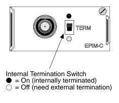
The link distance is up to 185 meters on the thin-net coaxial cables.
